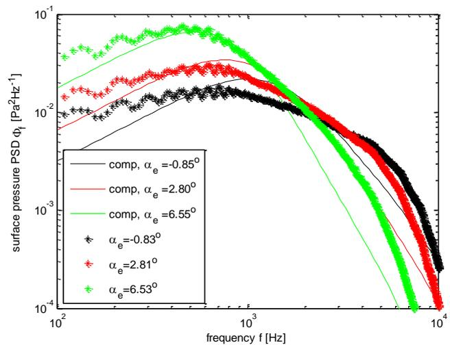
Figure 2: Improved model with surface blockage correction.
