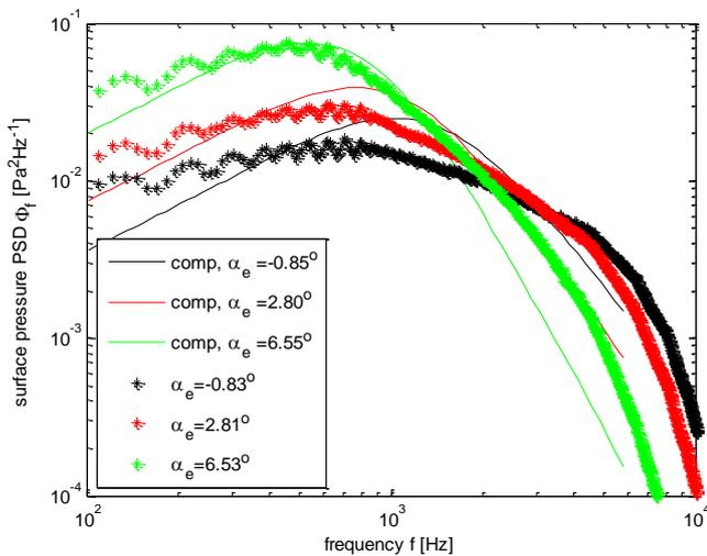
Figure 1: Improved model without surface blockage correction.
