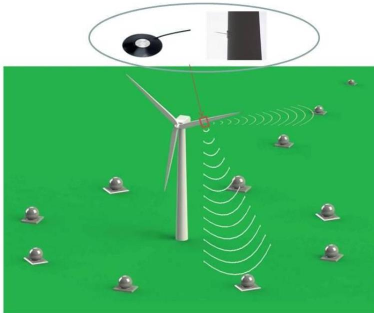
Figure 1: The experimental setup comprises a 500 kW turbine; 8 microphones on the ground in a circle around the turbine; 6 surface mounted microphones on the blade; one pitot tube on the blade and a meteorological mast.
