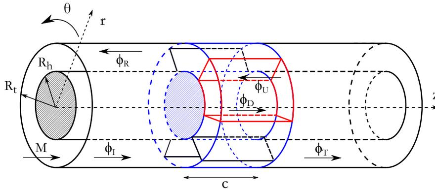
**Figure 1.** Annular cascade of vanes, modeled by zero-thickness flat plates, impinged by an incident acoustic wave of potential  $\phi_I$ . Scattered potentials for each subdomain are denoted  $\phi_R, \phi_D, \phi_U$  and  $\phi_T$ .
