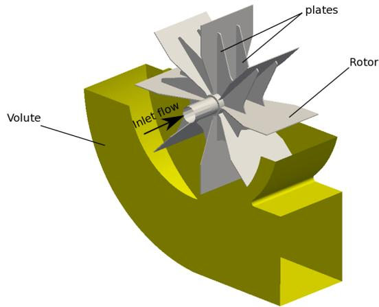
**Figure 2.** View of the radial rotor.
