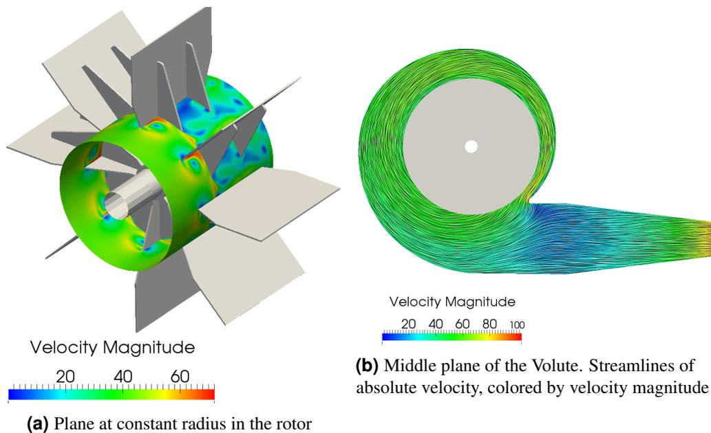
**Figure 5.** Velocity magnitude in the blower [m/s]
