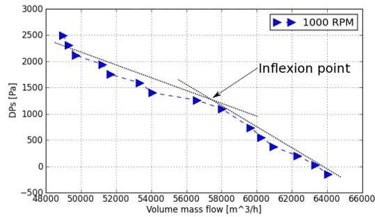
**Figure 4.** Performance curve of the blower – steady-state RANS simulations.
