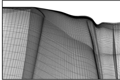
**Figure 3.** Typical casing contour to be optimized near the rotor tip
