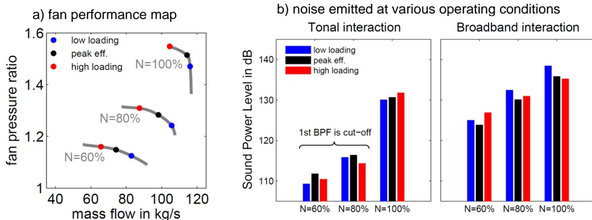
**Figure 2.** Assessment of the baseline fan performance a) and acoustic characteristics b)
