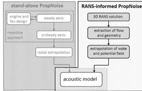
**Figure 1.** Structure of the acoustic prediction tool
