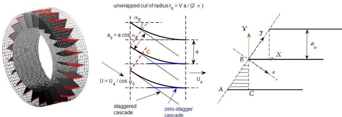
**Figure 1.** Typical axial-flow outlet guide vanes (left), unwrapped two-dimensional cascade representation (middle) and reference frames for Whitehead's formulation (right, opposite stagger angle).
