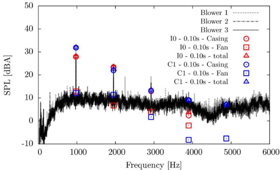
**Figure 3:** Noise spectra comparisons between experiments and simulations (red: incompressible and blue: compressible).
