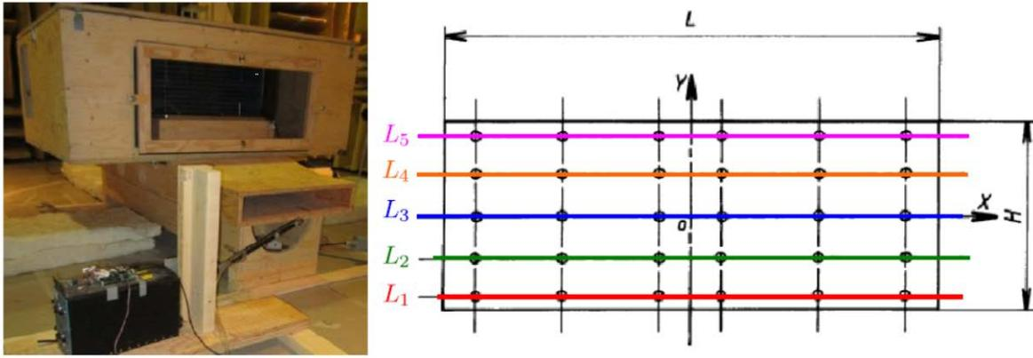
a) Experimental measurements of the velocity distribution over the outlet sections.
