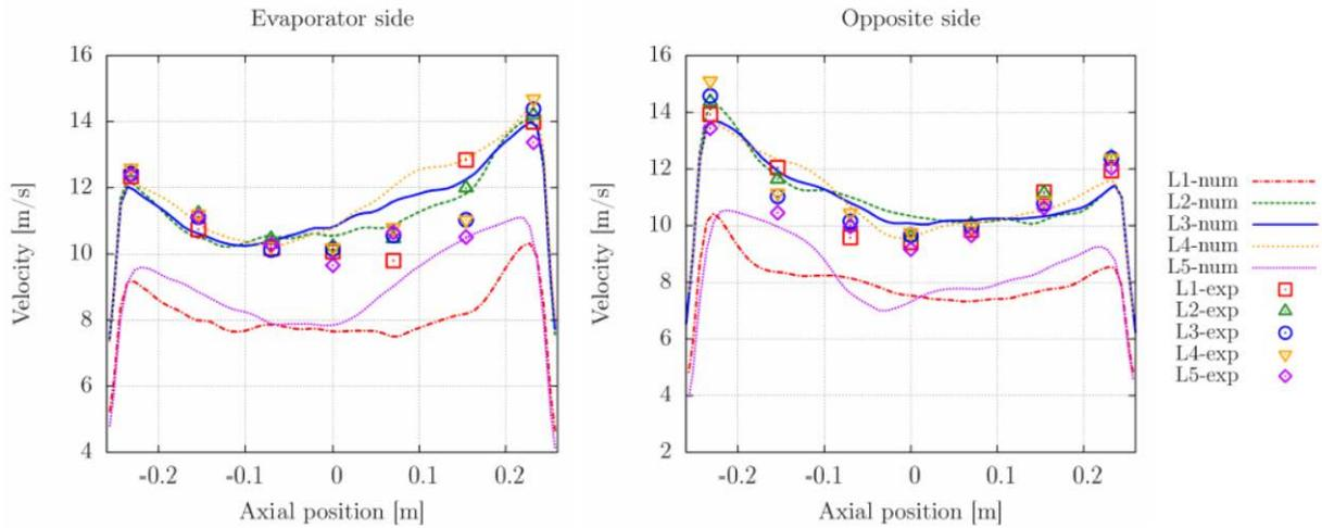
(b) Velocity distribution at the mock-up outlets from the Baseline simulations.
