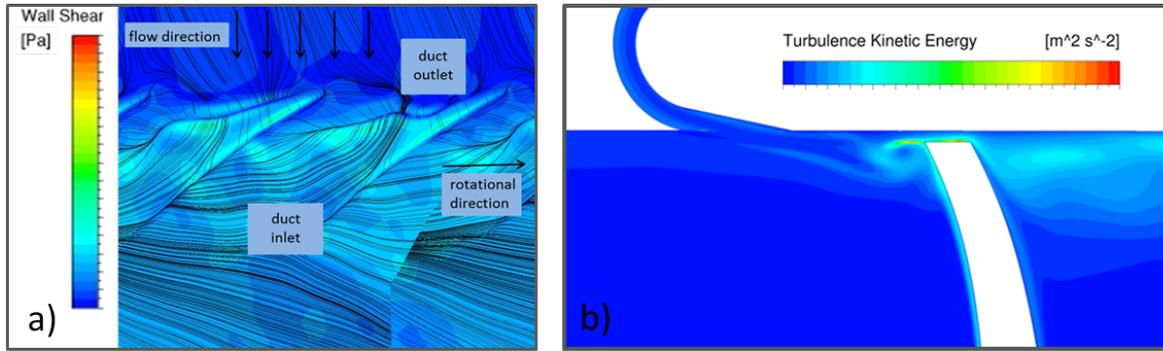
**Figure 1.** a) Path of Rotor Tip Gap Vortex at Shroud, b) Impact of Tip Blowing Jet on the Formation of the Tip Gap Vortex
