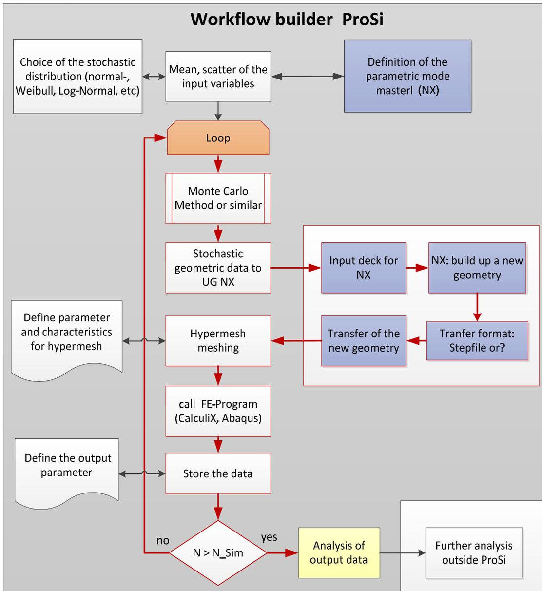
Within this paper the behaviour of a model panel is assessed with regards to its sensitivities and to enable local optimisation of the panel. To suit this purpose a process chain was developed and embedded into a Monte Carlo Simulation (MCS). As input parameters geometrical parameters, temperatures the manufacturing tolerances and their optimization ranges are used. First the behaviour of the nominal data are checked with manufacturing
