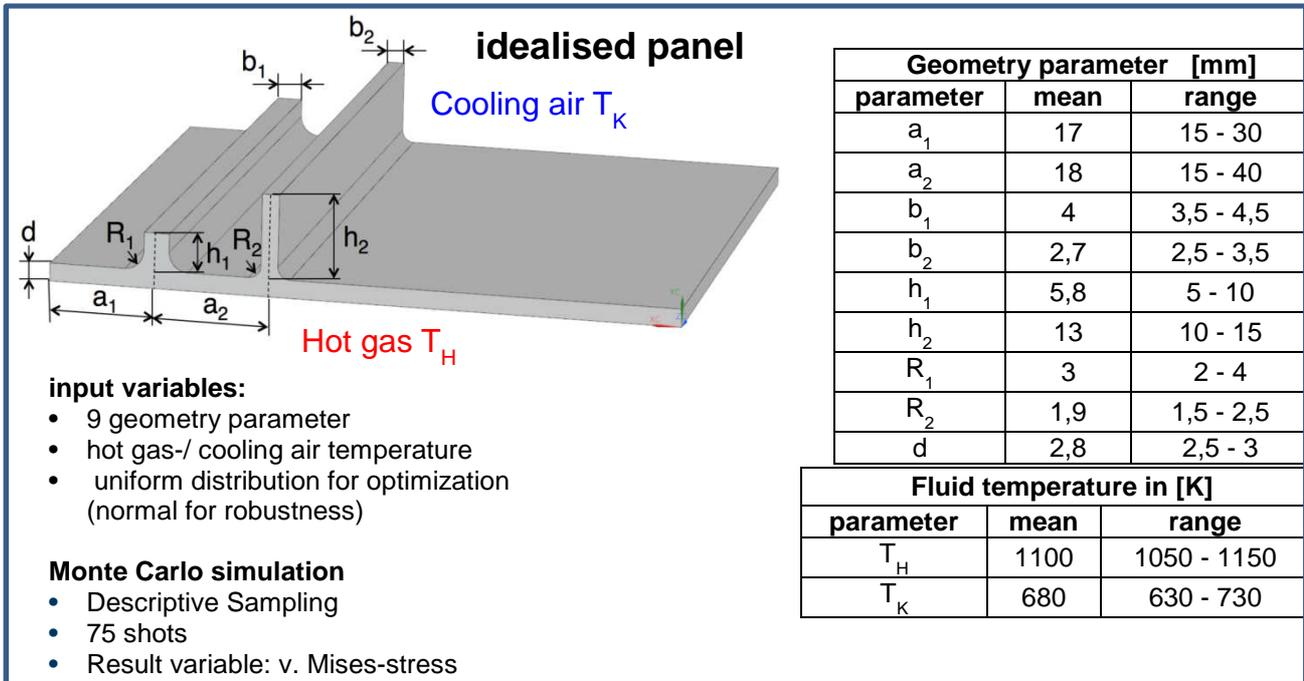
The calculations are carried out with ProSi as a workflow builder using NX for CAD and CalculiX for CAE. The output parameters such as stress are no longer deterministic, they are distributed with a mean value and a scatter. The closer the scatter the more robust the solution. This is shown in the results figure below.
