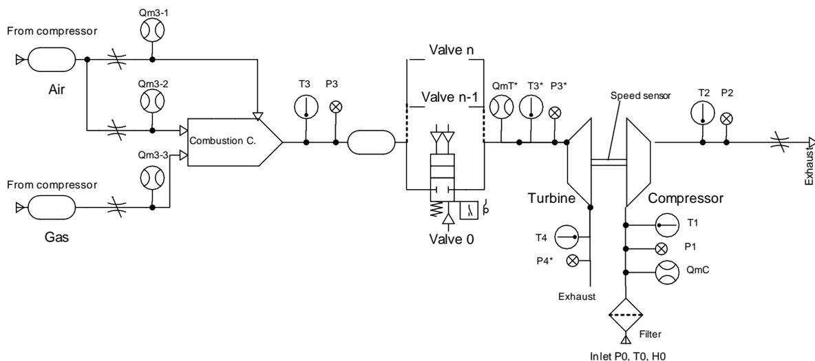
Figure 1. Test bench architecture
