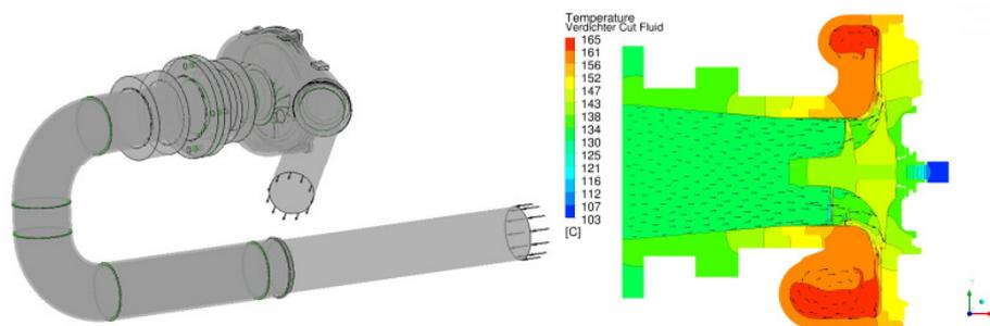
**Figure 3:** CHT model of high pressure compressor
