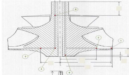
**Figure 2.** Position of thermocouples on compressor wheel
