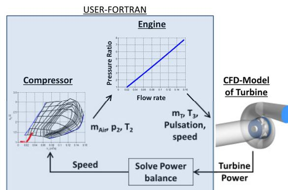
**Figure 1:** Schematic of Load Step Simulation
