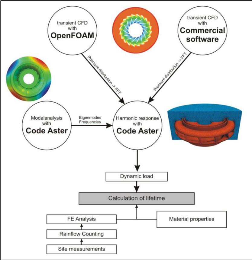
**Figure 1.** Method of component life time investigation
