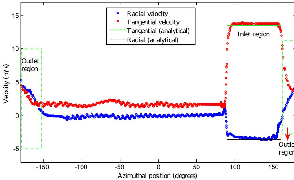
**Figure 4.** Comparison of radial and tangential velocities (CFD and analytical) at the impeller boundary for the new nozzle
