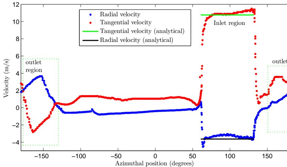
**Figure 3.** Comparison of radial and tangential velocities (CFD and analytical) at the impeller boundary for the existing nozzle
