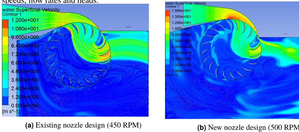
**Figure 2.** Water velocity contours with streamlines superimposed for two nozzle designs at maximum efficiency.
