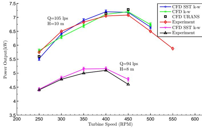
**Figure 1.** Comparison of CFD predicted and measured turbine power outputs at different impeller speeds, flow rates and heads.
