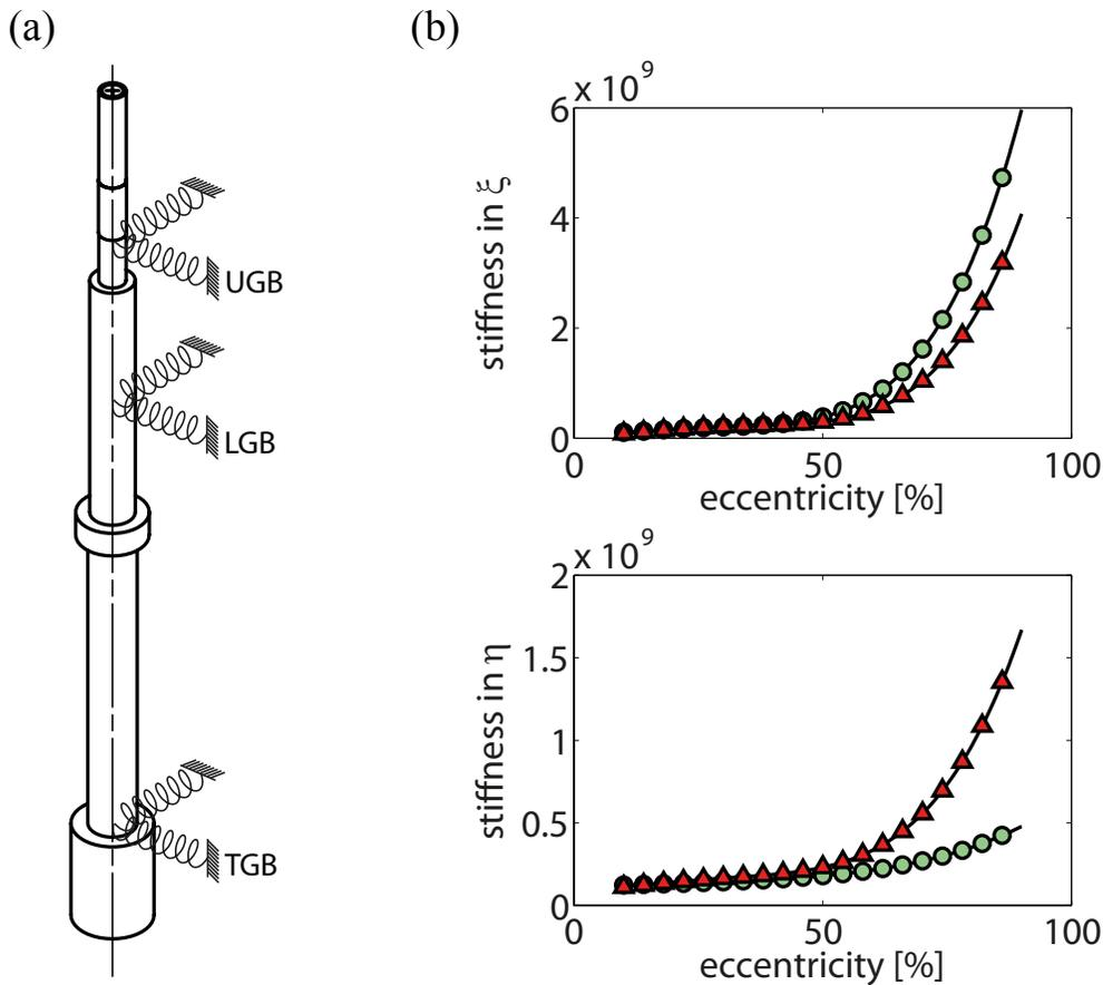
**Figure 1.** (a) Model of hydropower turbine supported by three tilting pad journal bearings (b) Bearing stiffness of the UGB for LOP ( $\circ$ ) and LBP ( $\Delta$ ) in the  $\xi$  and  $\eta$  directions (rotating frame) as function of eccentricity for a rotating speed  $\Omega = 2350$  RPM
