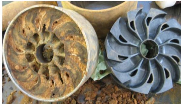
**Figure 1.** Example of Ochre Deposits on the Diffusor of a Submersible Pump
