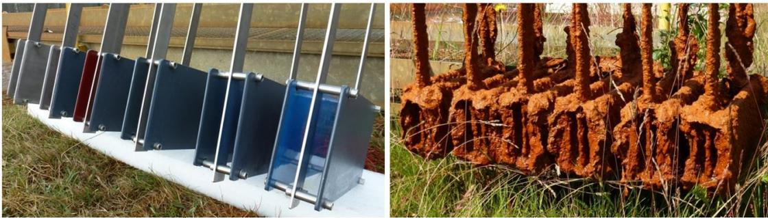
**Figure 2.** Sample Carriers Clean (left) and Iron Clogged (right)
