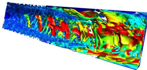
**Figure 1:** Isosurface of the velocity invariant  $Q=1$  colored by viscosity ratio 0-1000 for a mesh with about 30 million elements
