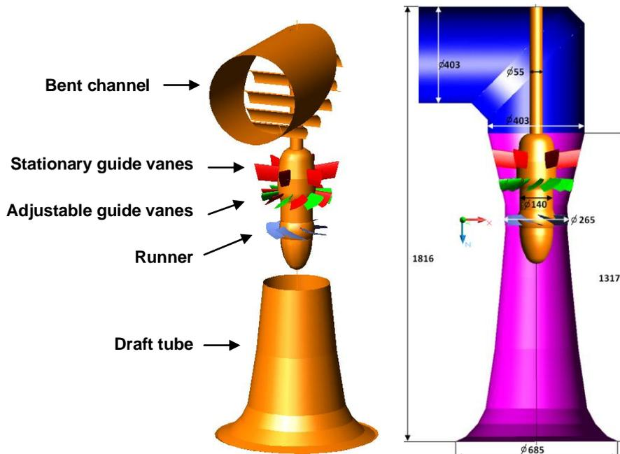
Figure 1. A vertical model Kaplan turbine – the object of the experimental tests.
