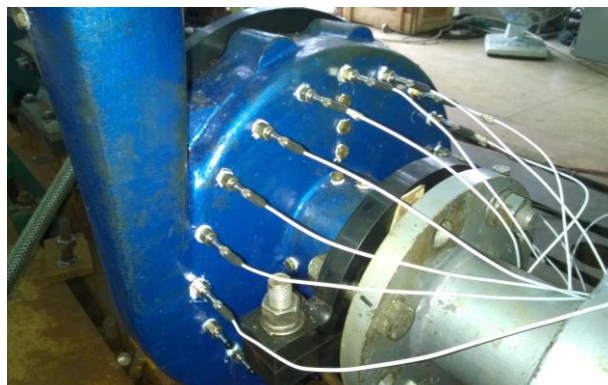
Figure 2. Pressure pulsation and vibration test
