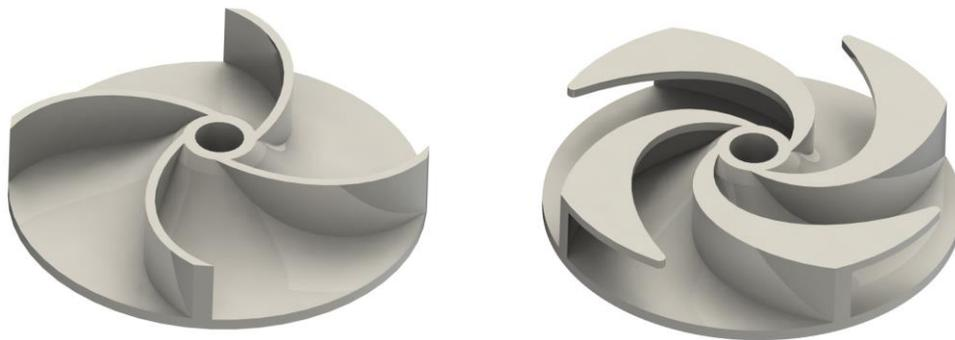
**Figure 1.** Schematic View of the Impellers of a Vortex Pump without Winglets (left) and with Winglets (right)
