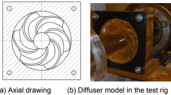
**Figure 1.** Diffuser Geometry and Solid Model
