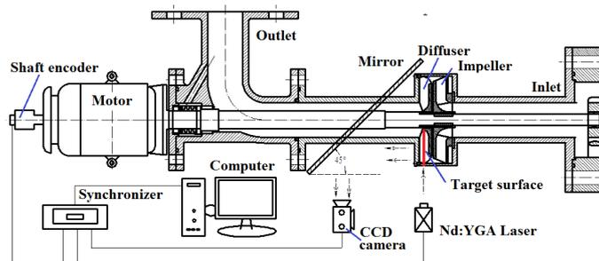
**Figure 3.** Schematic of Test Rig and PIV System
