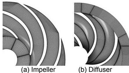
Figure 5. Sketch of the Structured Grid
