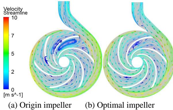
**Fig.5** Comparison of velocity distribution in the impeller under design condition
