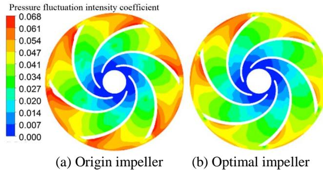
**Fig.6** Pressure fluctuation intensity distribution in the impeller
