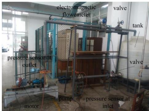
**Fig. 3** Pump open test rig
