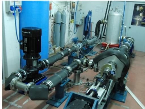
**Figure 1.** The cavitating pump rotordynamic test facility
