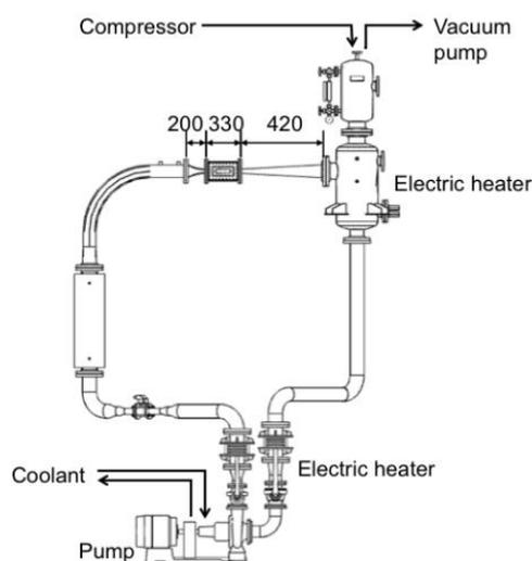
**Figure 1.** Overview of high temperature and high pressure water tunnel in Institute of Fluid Science of Tohoku University.
