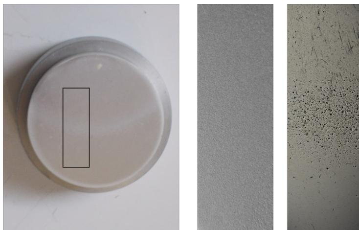
**Figure 2:** A damaged specimen after 30 minutes of exposure to cavitation.
