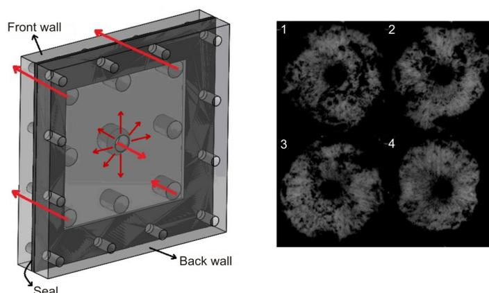
**Figure 1:** Test section (left) with a typical cavitation structures (right).
