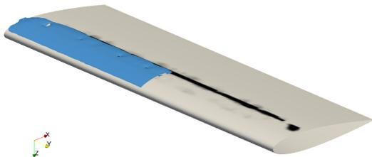
**Figure 1.** Cavitation erosion at  $\sigma = 1.19$
