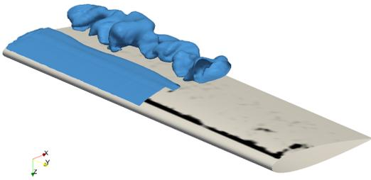
**Figure 2.** Cavitation erosion at  $\sigma = 0.95$
