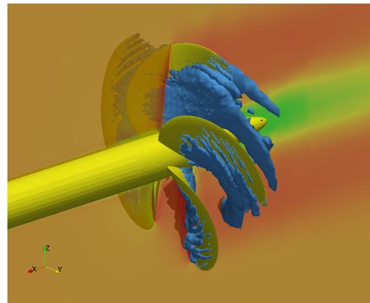
**Figure 3.** Cavitating propeller from perspective view
