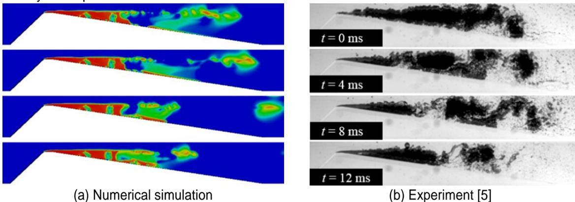
**Figure 2.** Typical example of simulation of 2-D convergent-divergent nozzle flow
