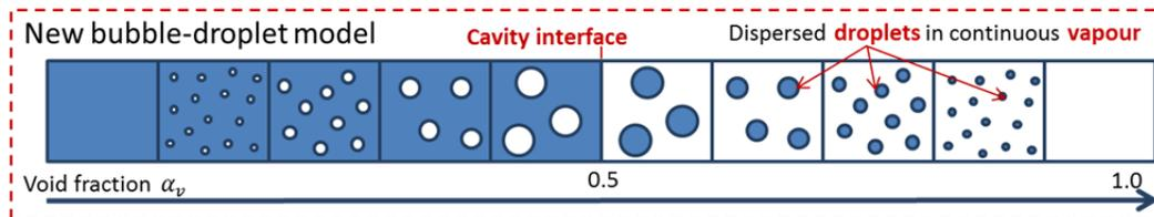
**Figure 1.** Conceptual drawing of bubble-droplet model
