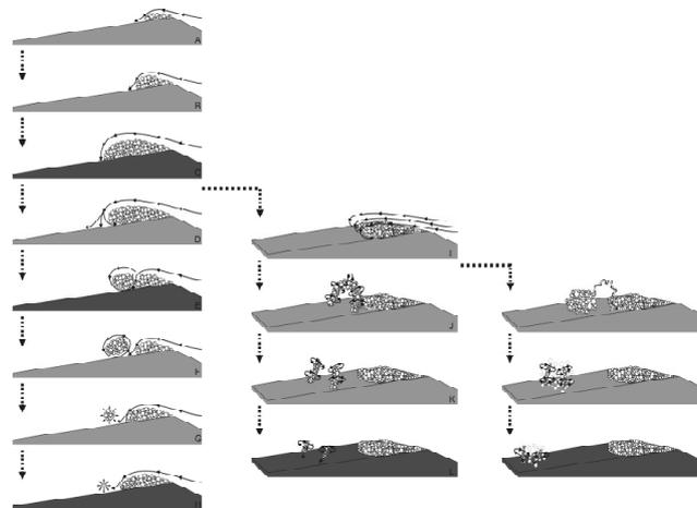
**Figure 1:** Schematic representation of observed mechanisms that lead to occurrence of cavitation erosion. The instants of damage appearance are denoted by the darker colour [2].
