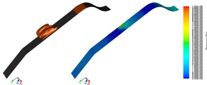
**Figure 2:** Pressure peak, with an amplitude exceeding 10 bar, occurring during a small scale cavitation structure collapse.
