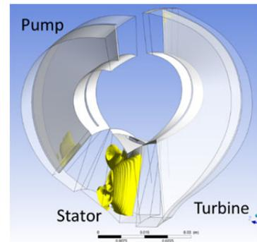
(b) Cavitation around 20% torque drop
