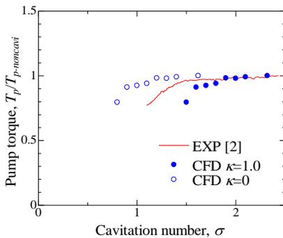
(a) Pump torque characteristics
