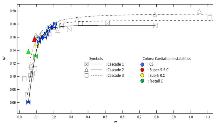
**Figure 1.** The head performance and occurrence region of cavitation instabilities of the present cascades with and without random slit
