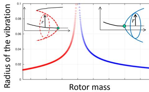
**Figure 2** Influence of the rotor mass to the bifurcation type of oil whirl or oil whip
