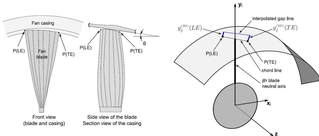
**Figure 2.** Geometry of the contact region and 3D view of the clearance values interpolated along the chord line
