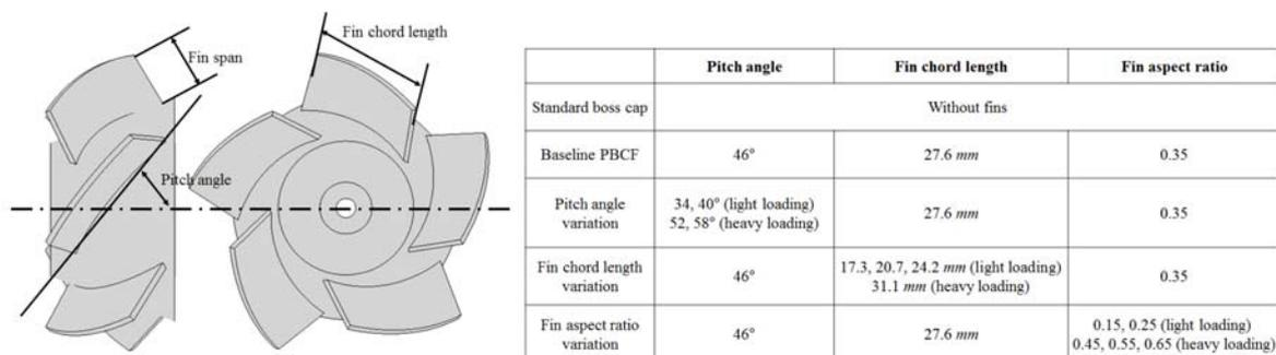
**Figure 1.** Design Parameters of PBCF and test conditions
