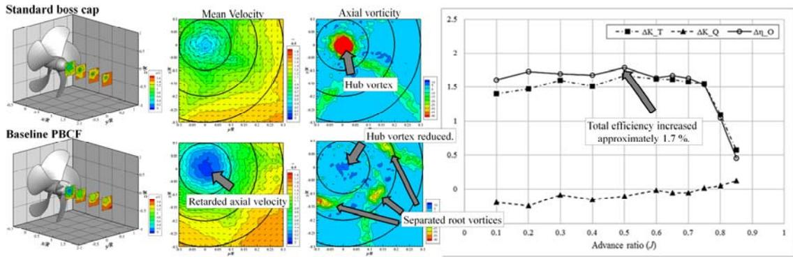
Figure 2. Wake Field and Global Force Measurement Results
