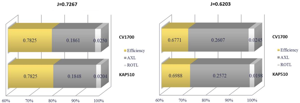
**Figure 2:** The energy coefficient analysis for a conventional propeller CV1700 (upper) and a Kappel propeller KAP510 (lower) at  $J=0.7267$  (Left) and  $J=0.6203$  (Right)
