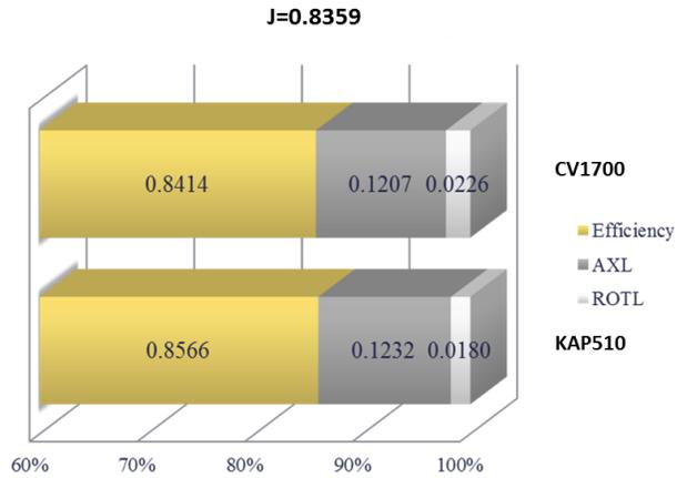
**Figure 1:** The energy coefficient analysis of a conventional propeller CV1700 (upper) and a Kappel propeller KAP510 (lower) at  $J=0.8359$
