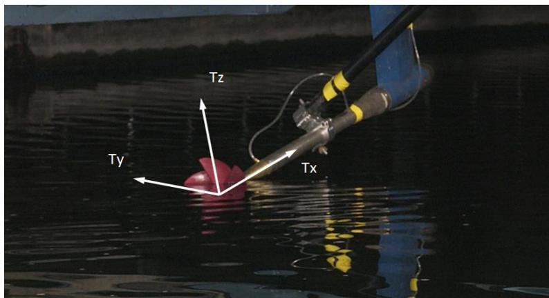
*An example of a test set-up and the coordinate system of the forces*
