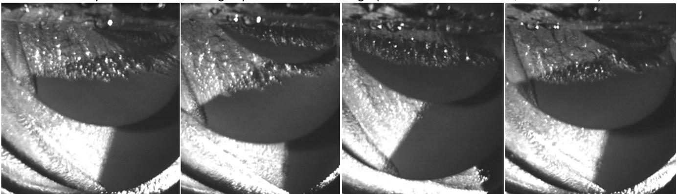
Sequence of blade entrance (partial ventilation, blade submersion 0.6R, inclined shaft)
