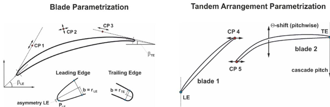
Figure 1. Cascade Parametrization
