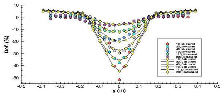
Figure 2 Comparisons of velocity deficit distribution between simulated results and measured data
