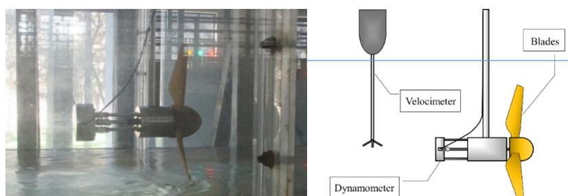
Figure 1 A sketch of the scale turbine and the gauge system
