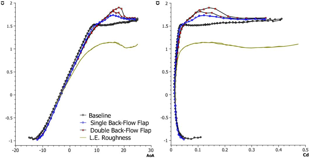
**Figure 2.** Wind tunnel test results of various backflow flap configurations.
