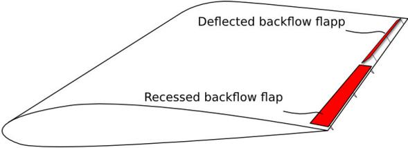
**Figure 1.** Basic representation of a deflected and a recessed flap on a blade section.
