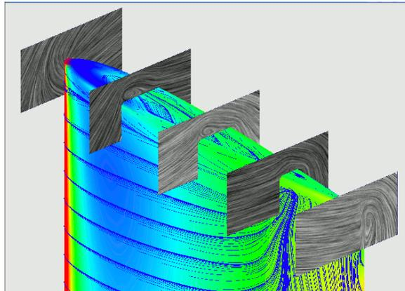
Figure 3. Limiting streamlines and tip vortex around a blade.
