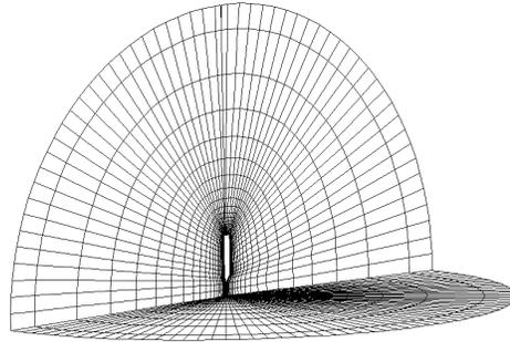
Figure 1. 3-D computational O-O grids of the 2 blades wind turbine.
