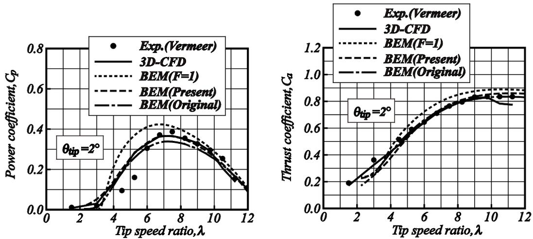
Figure 2. Power and Thrust Coefficient for CFD, BEM and the experiment results.
