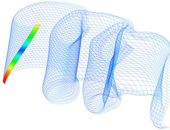
**Figure 1.** Detail of free evolving wake of single blade VAWT, QBlade screenshot
