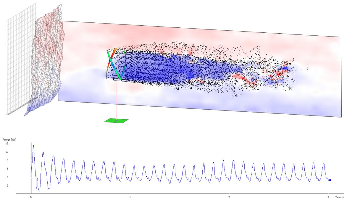
**Figure 2.** A Visualization of unsteady LLT simulation in turbulent windfield, resulting torque over time
