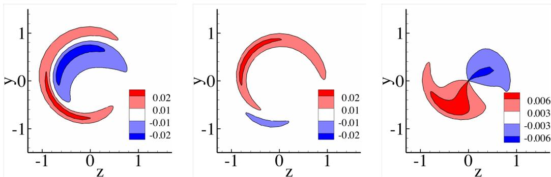
**Figure 2.** Components of the optimal inflow perturbation in streamwise, vertical and azimuthal directions from left to right.
