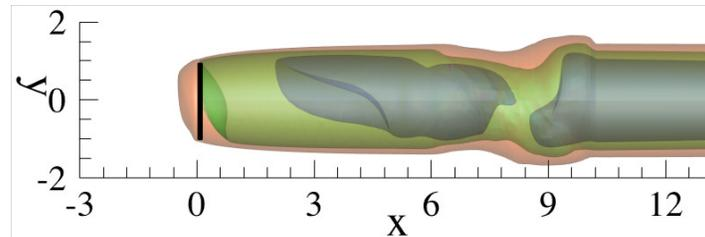
**Figure 1.** Iso-surface of streamwise velocity 0.3, 0.5, 0.8 (normalised by free-stream velocity) of the optimally perturbed flow. The optimal perturbation is introduced from the inflow boundary located at  $x = -3$ ; the location of the disc model is indicated by the thick line.
