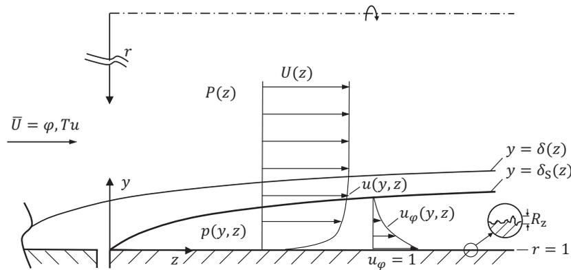
**Figure 1.** Flow at the inlet of a rotating pipe.
