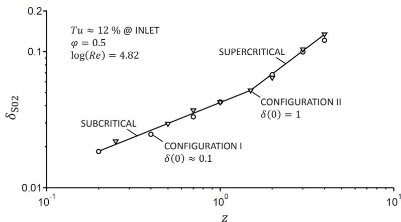
**Figure 2.** Instability of the swirl boundary layer with a turbulent flow at the inlet of a rotating pipe.
