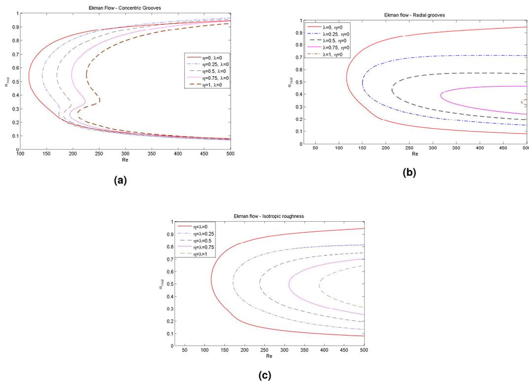
**Figure 1.** Neutral curves of Ekman flow over rough disks. (a) anisotropic roughness - concentric grooves, (b) anisotropic roughness - radial grooves, and (c) isotropic roughness
