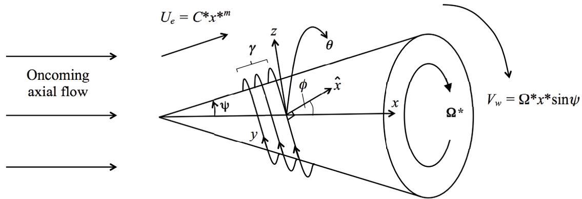
**Figure 1.** Diagram of the spiral vortex instability on a rotating cone placed in an oncoming axial flow, showing coordinates in the  $\hat{x}$ - and  $\hat{y}$ -logarithmic spiral directions, as well as the corresponding vortex wavenumber,  $\gamma$ , and vortex waveangle,  $\phi$ .
