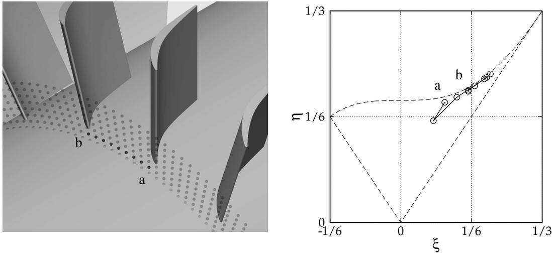
**Figure 1.** Characterization of turbulence anisotropy according to the invariant theory by Lumley [7] at  $h/H = 5.9\%$  upstream of the blades leading edges.
