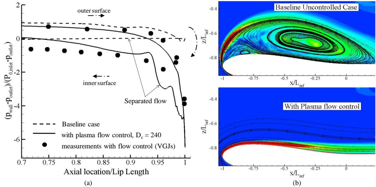
Figure 2: (a) Non-dimensional pressure distribution over the intake lip (b) Contours of vorticity magnitude for the baseline case and with plasma actuator,  $D_c = 240$
