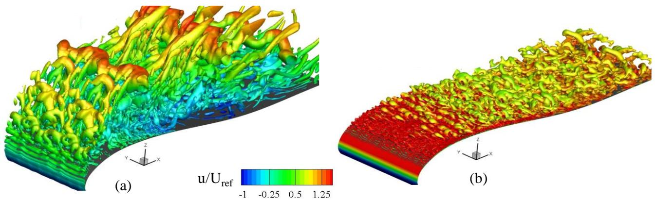
Figure 3: Iso-surfaces of  $Q$  contoured with axial velocity a) for the baseline case and b) with plasma actuator,  $D_c = 240$
