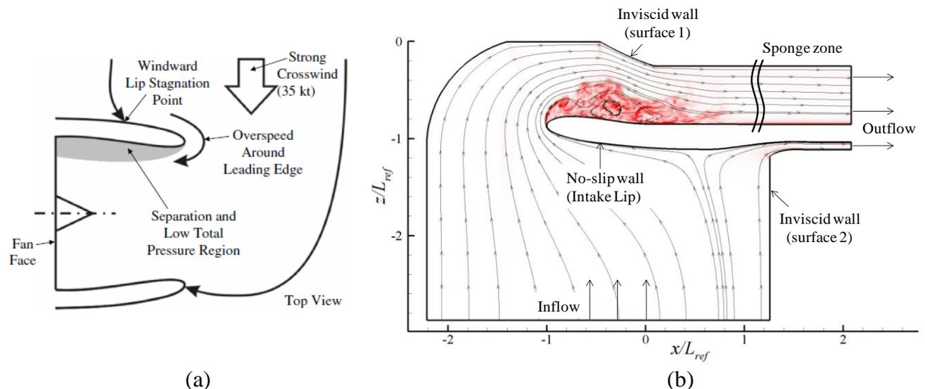
Figure 1: a) Schematic showing typical off-design crosswind condition [1] b) Computational domain and boundary conditions (contour of vorticity magnitude and streamlines are shown to highlight the separated region around the intake lip)
