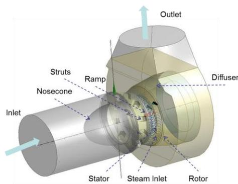
Figure 1. FCC Hot gas expander fluid domain
