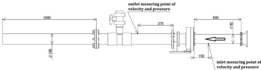
Fig.1 Radial fan test facility
