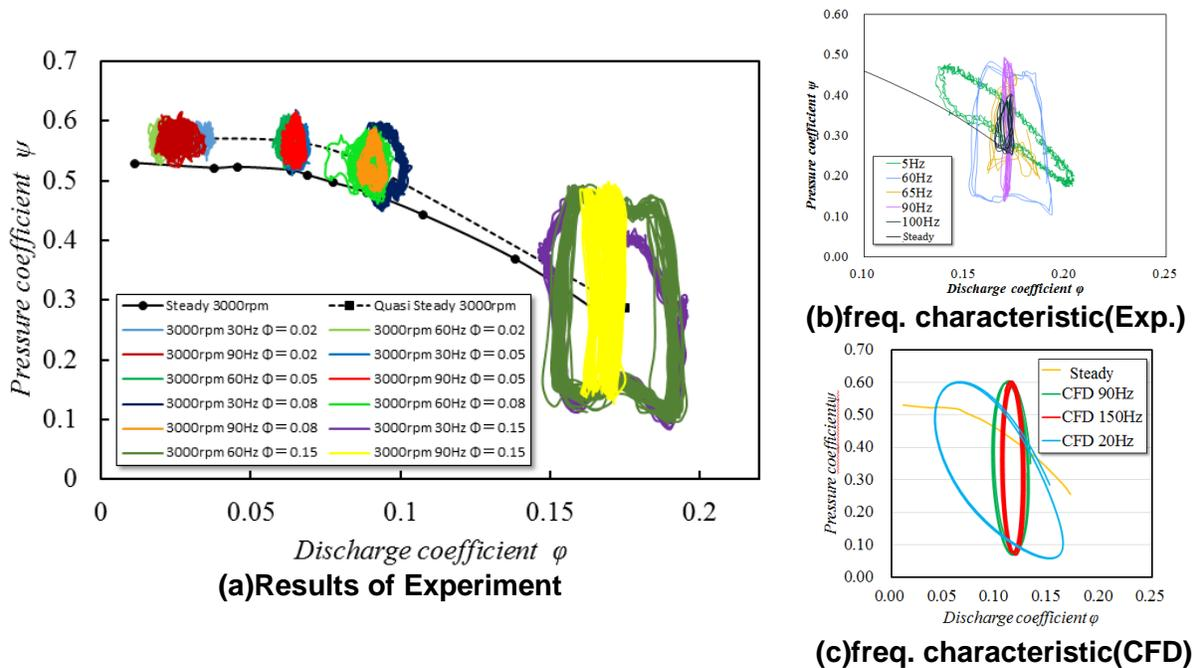
Fig. 3 performance curve under unsteady flow
