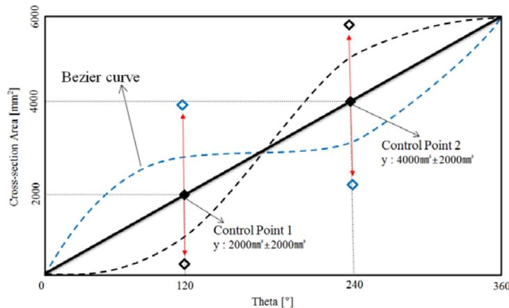
**Figure 2.** Area distribution with the theta angle of the volute
