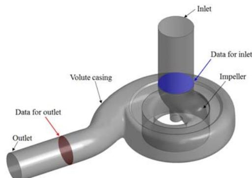
Figure 1. Single-channel pump for wastewater treatment
